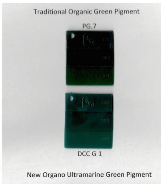
Figure 7 – Shade Comparison of Green Organo-Ultramarine Pigment vs Pigment Green 7
