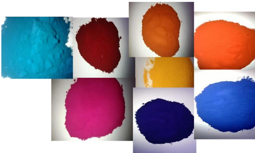
**Figure 2 – examples of colour range of the new Organo-Ultramarine pigments**
