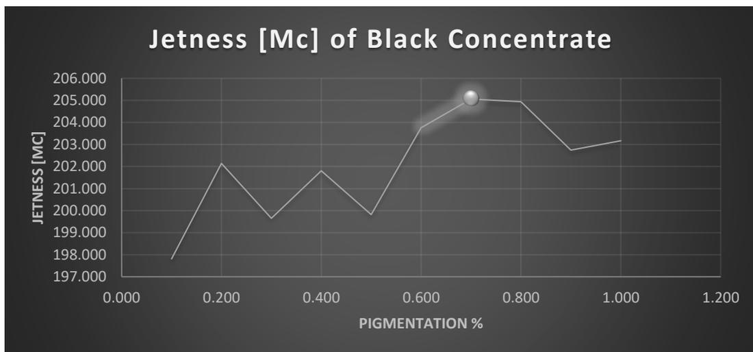
**Figure 1.** Jetness of the commercial carbon black concentrate, varying in pigment loading
