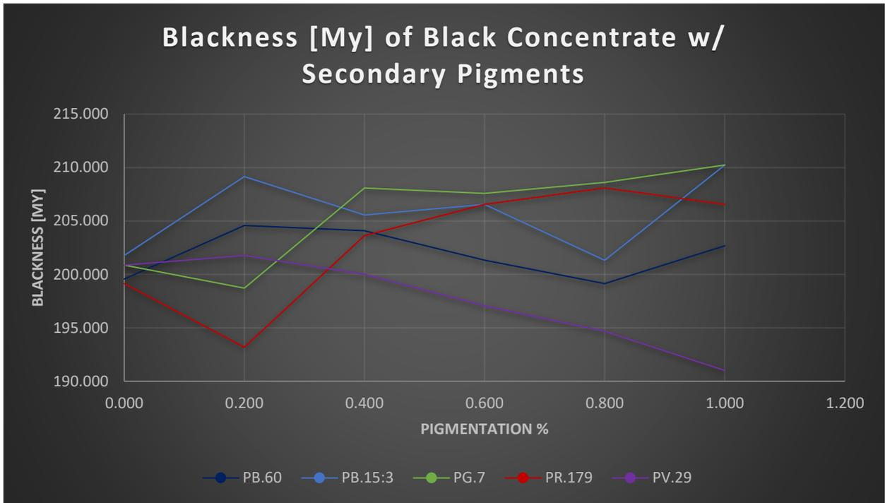
**Figure 3.** Comparison graph of Blackness of the commercial carbon black concentrate with each secondary color.
