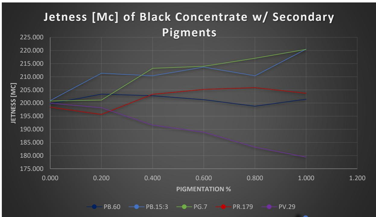
**Figure 2.** Comparison graph of Jetness of the commercial provided carbon black concentrate with each secondary color.
