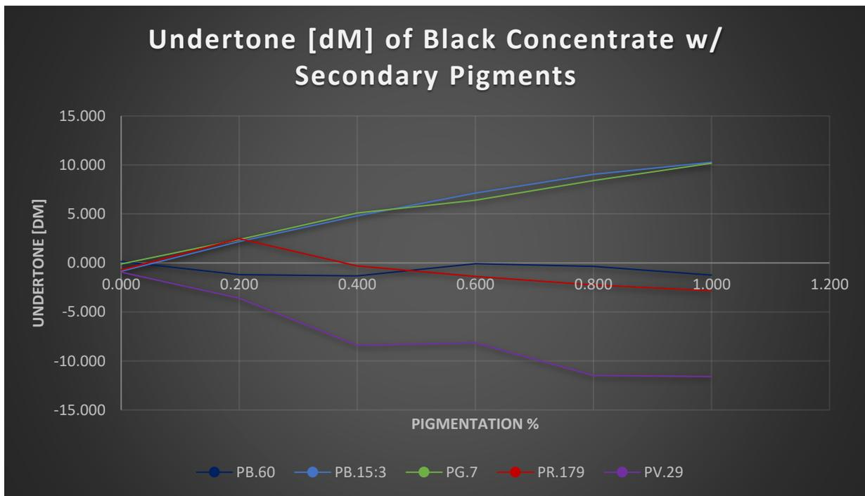
**Figure 4.** Comparison graph of Undertone of the commercial carbon black concentrate with each secondary color.
